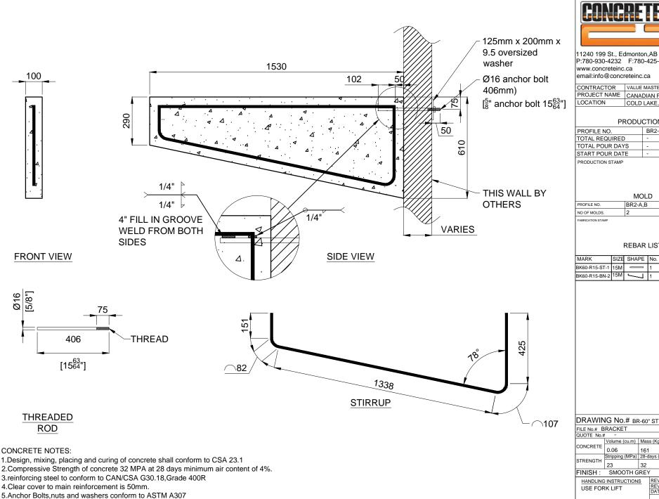
6.Weld to conform to CSA W59, 2003 comply with the CSA W47.1 Division 2.Use minimum 6mm fillet weld.
